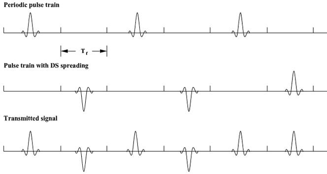
Fig. 8. The transmitted signal along with its component signals used in [40].
