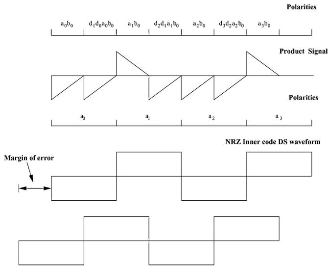
Fig. 16. Illustration of the margin of error tolerable in the despreading of the inner code in the first stage.
