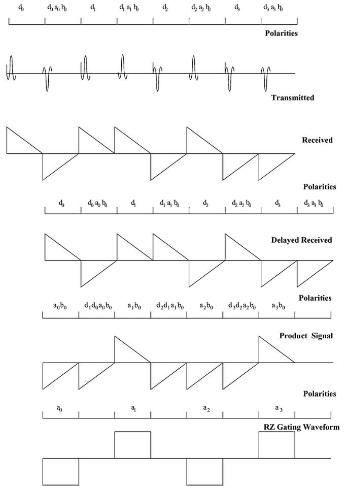
Fig. 15. Illustration of the delay and multiply operation on the noiseless received signal.
