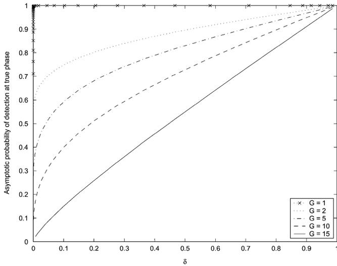
Fig. 12. The AROC for a detection based acquisition system using EGC for different values of EGC window size  $G$ .
