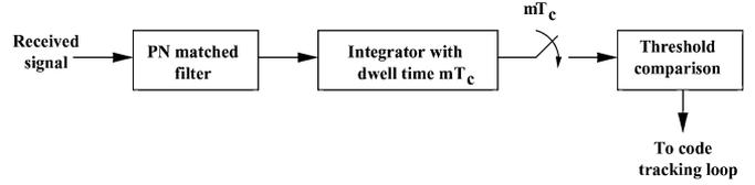
Fig. 4. Block diagram of the acquisition scheme proposed in [26].
