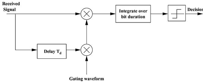
Fig. 14. Block diagram of the autocorrelation receiver.
