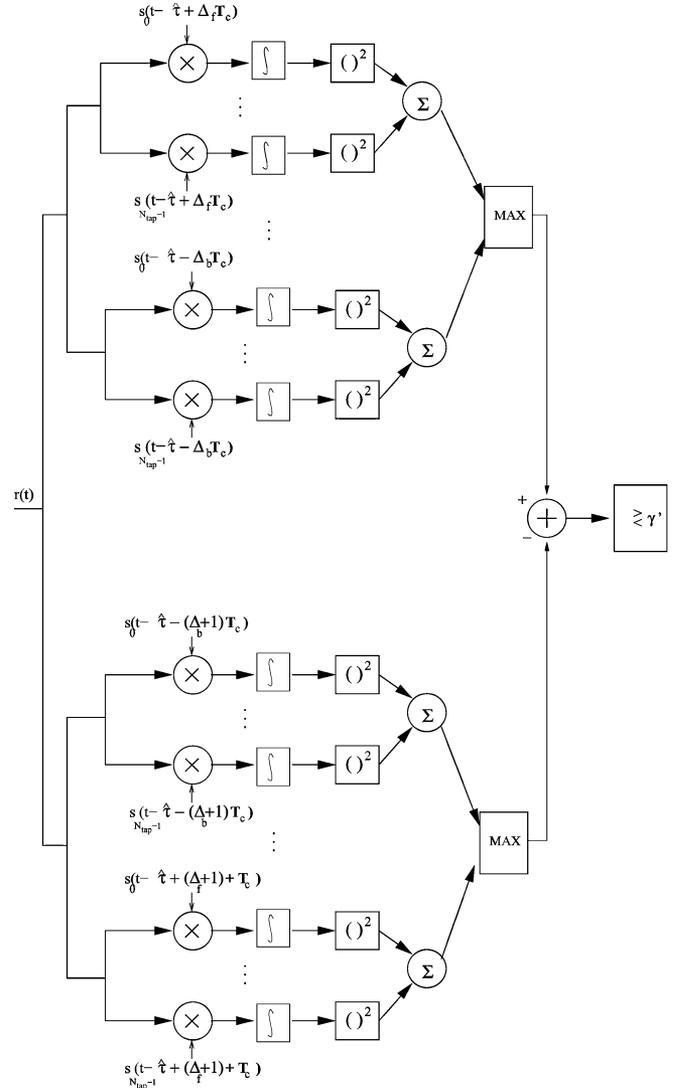
Fig. 13. Generalized likelihood ratio test for evaluation of phase  $\hat{\tau}$ . The upper and lower MAX operations evaluate the maximum of  $\sum_{k=0}^{N_{\text{tap}}-1} C_k^2(\nu)$  over  $\nu \in \mathcal{S}(\hat{\tau})$  and  $\nu \notin \mathcal{S}(\hat{\tau})$ , respectively.
