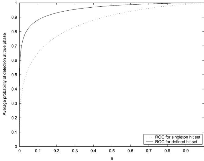
Fig. 11. The ROCs when the threshold is set for a singleton hit set containing only the true phase and for a hit set defined in (12) with  $\lambda_n = 10^{-3}$ .
