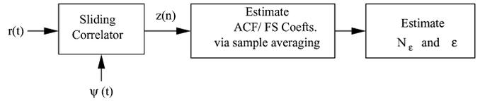
Fig. 9. Autocorrelation function (ACF) of correlator outputs  $z[n]$  or its Fourier series (FS) coefficients estimated via sample averaging and used to estimate timing offset.
