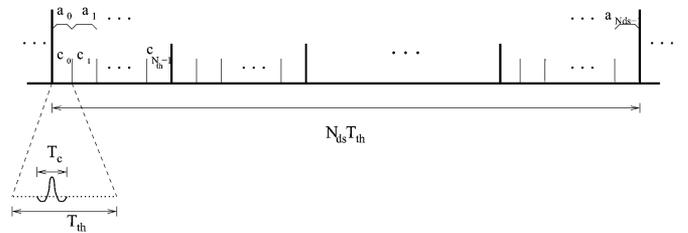
Fig. 6. The hybrid DS-TH signal format used in [39].
