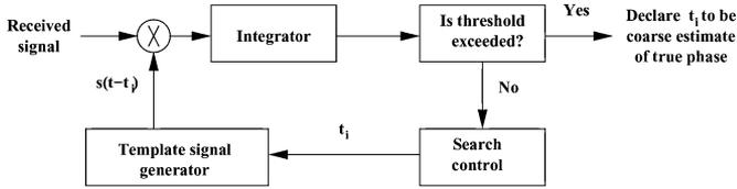
Fig. 3. Block diagram of the acquisition scheme proposed in [25].
