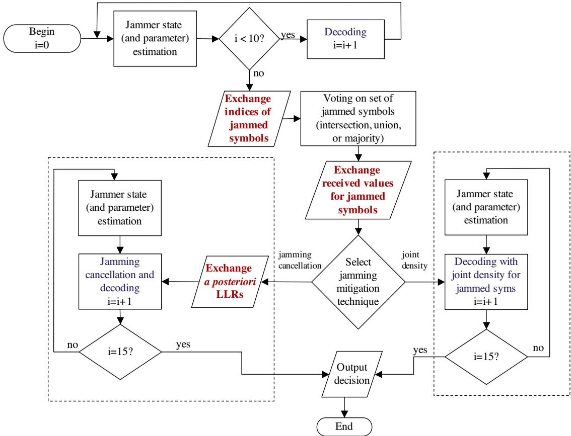
Fig. 3. Flowchart for collaborative jamming mitigation techniques.
