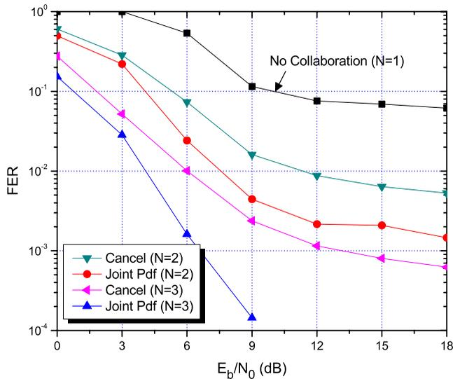
Fig. 6. Performance of the jamming mitigation schemes for perfect CSI ( $E_b/N_J = -6$  dB,  $\rho = 0.6$ ,  $E\{T_J\} = 50$ ).
