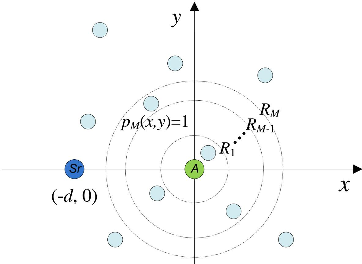
Fig. 3. Illustration of optimal forwarding resolution protocol in geographic transmission.  $S_r$  = source node.  $A$  = access point.
