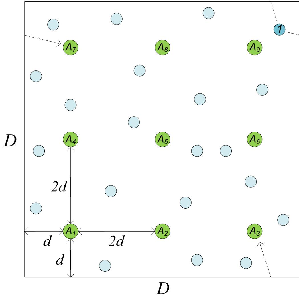
Fig. 1. Example of mesh network layout with 9 access points.  $A_i = i$ -th access point.
