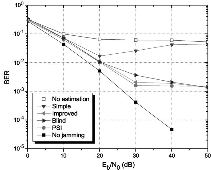
Fig. 9. Performance of jamming detection with various initial estimates in quasi-static fading channels ( $E_b/N_J = 8$  dB,  $\rho = 0.4$ ).
