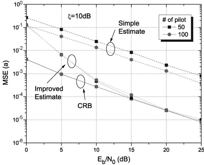
Fig. 3. Comparison of MSE for simple and improved estimates of channel gain  $a$ .
