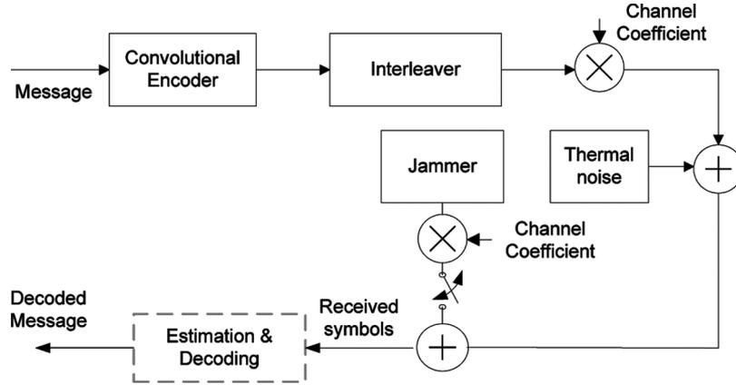
Fig. 1. System model for estimation and decoding in partial-time Gaussian jamming.
