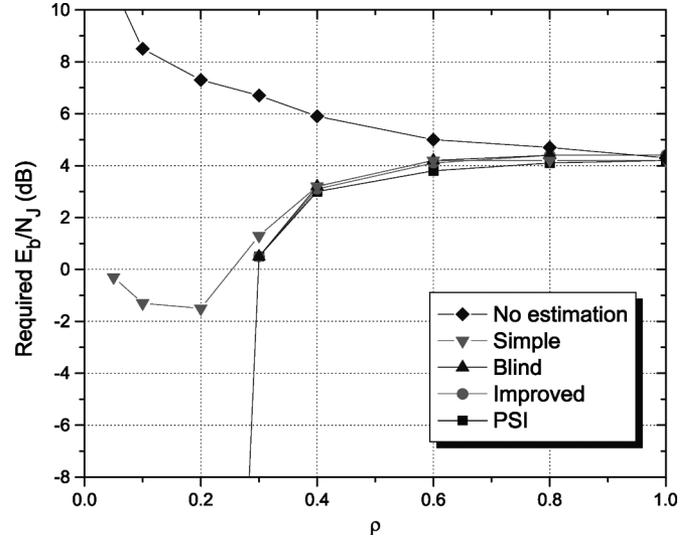
Fig. 8. Required  $E_b/N_J$  to obtain a FER of  $10^{-2}$  ( $E_b/N_0 = 15$  dB).
