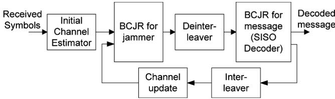
Fig. 2. Iterative estimation and decoding.
